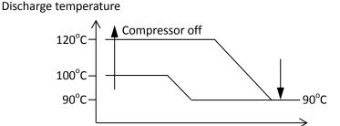
When the discharge temperature rises above 120°C the system displays P4 protection and all units stop running. When P4 protection occurs 3 times in 100 minutes, the H6 error is displayed. When an H6 error occurs, a manual system restart is required before the system can resume operation.
