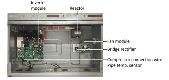
Figure 5-1.3: 20-32HP top layer of electric control box
