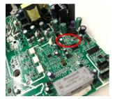
4. Check the power supply for the compressor inverter module, port CN41 on filter board, the normal voltage should be DC310V; check the high pressure switch connection port CN61 on filter board, the normal resistance should be zero; Check the single phase bridge and fuse on filter board; check the connection cable from ODU main PCB port CN82 to filter board port CN30 which is DC310V power control port.
