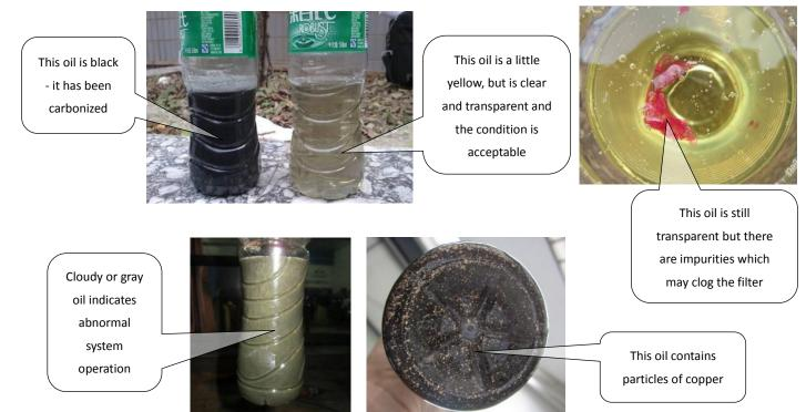
Figure 6-2.11: Effects of spoiled compressor oil
