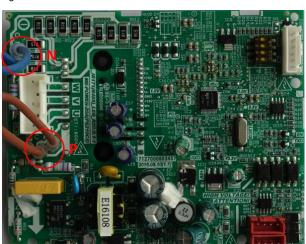
Figure 6-2.12: Fan module P N terminals
