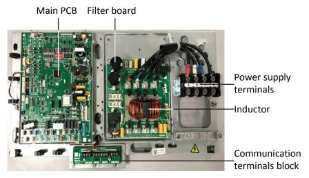
Figure 5-1.2: 8-18HP bottom layer of electric control box
