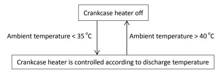
Figure 3-3.2: Crankcase heater controlled according to discharge temperature
