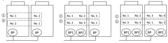
Figure 3-4.3: Compressor priority and rotation – three outdoor units
