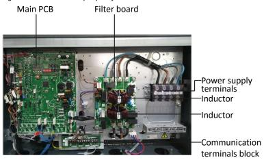
Figure 5-1.4: 18-30HP bottom layer of electric control box
