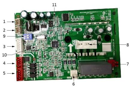
Table 5-4.1: Fan module PCB ports
