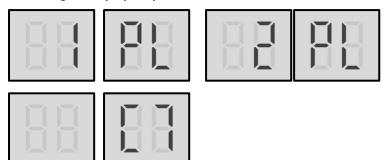
'x' is a placeholder for the compressor system (compressor and related electrical components), with 1 representing compressor system A and 2 representing compressor system B.
