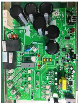
Figure 6-2.1: P and N terminals on Inverter module
