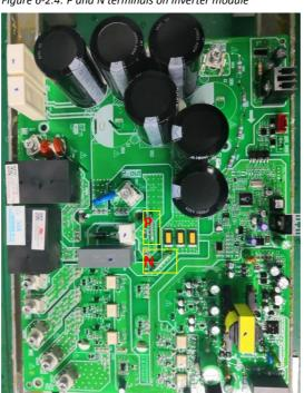
Figure 6-2.4: P and N terminals on Inverter module
