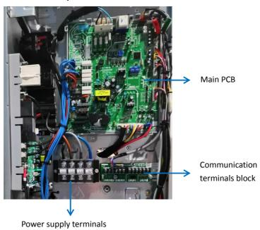
Figure 5-1.2: Rear view of electric control box
